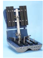
All-new STAN manikin for seat testing.
